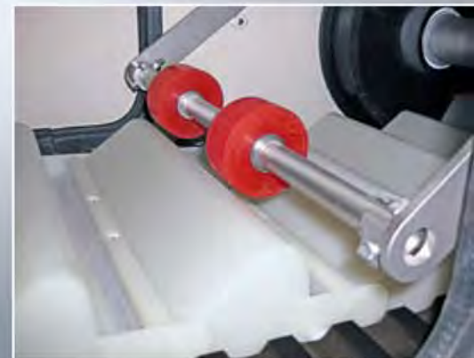
Pendulum bucket knocker to assist product discharge
