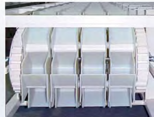
Multiple bucket belt at the tensioning unit
