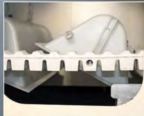
Buckets are emptied by the tilting mechanism
